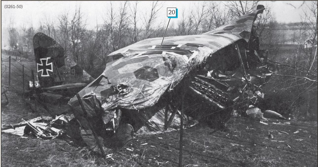
The camouflage paint has flaked off the crumpled wing exposing the bleached 'white' linen (m) fabric beneath.
