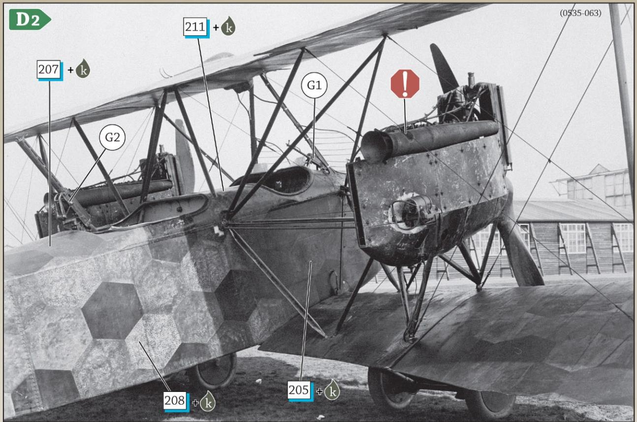
Rear view of the starboard engine nacelle and fuselage from captured AEG G.IV 1125/16 **D**. Note the uncommon mix of LMG 14 (G2) and LMG 14/15 (G1) Parabellum machine guns for the front and rear armament.
