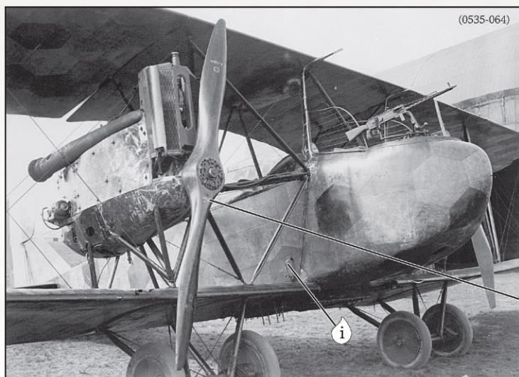
Front view of the starboard engine nacelle and nose from captured AEG G.IV 1125/16 **D**. Note the white **i** fuel lines leading from the side of the fuselage into the bottom wing and the addition of an RFC pitot head above the cabane struts.
