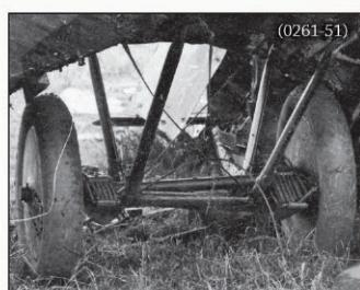
Undercarriage detail from an unidentified crashed AEG G.IV. Note the displaced axle and suspension spring details.
